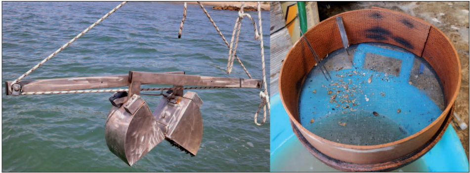
Figure 7 - Soft-bottoms infauna: Van Veen grab (left) and sorting (right) of the samples.
