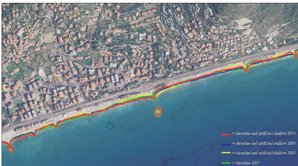
Figure 10 - The littoral of Borgio Verezzi (SV). Variation of the shoreline from 2007 to 2010.
