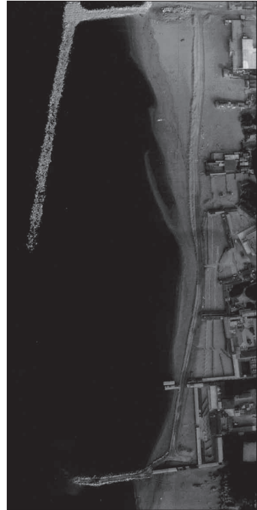
Figure 15 - Above: works executed on 19 05 1999 (Photo: DST-UNIFI archives); Right: structure status on 13 03 2000 (Photo: Corpo delle Capitanerie di Porto, Luni - Sarzana). Although the structure was designed with a submerged crest, it induced changes on beach morphology that had not been predicted by the project.
