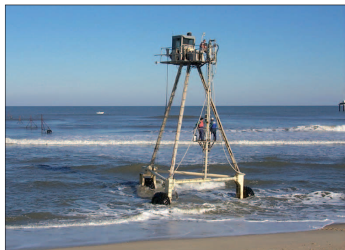
Figure 13 - Coastal Research Amphibious Buggy (CRAB) used for beach profile measurements at the U.S. Army Corps of Engineers Field Research Facility, Duck, North Carolina
