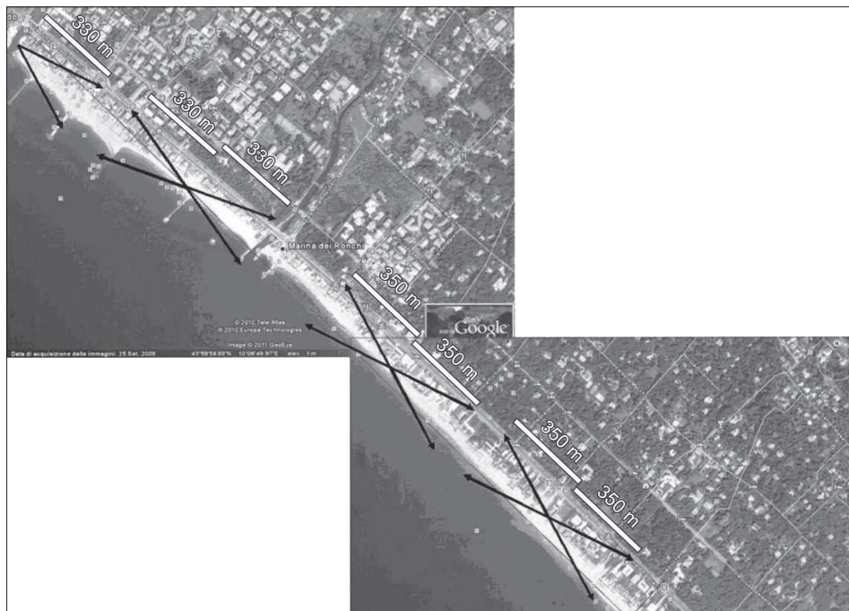
Figure 2 - Explicative scheme of the video monitoring network (modified from Google Earth).
