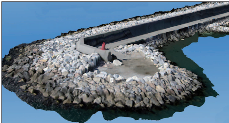
Figure 25 - Aerial photographic survey of a port with a small drone (Menci software).
