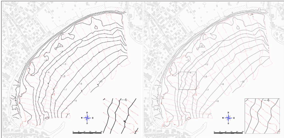
Figure 35 - Automatic generation of contour line for a SB survey. Normal (top), smoothed (below). Golfo di Campo (Elba Island - Italy).
